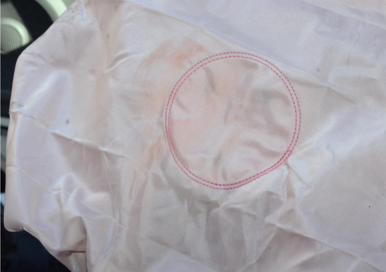
Deployed Driver Airbag showing contact with Driver Occupant
